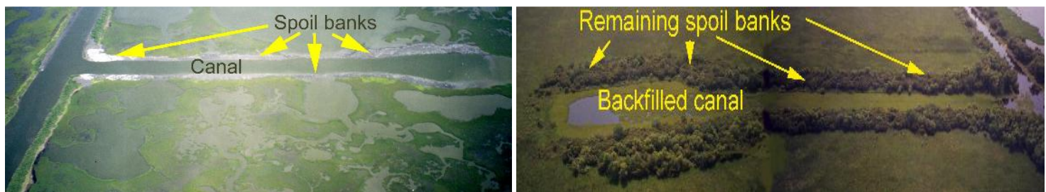
Figure 13: Backfilling canals (Ramasar, 2008)
