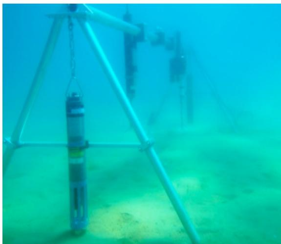
Figure 8: Sediment resuspension device. UC Davis
